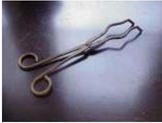
Name: tongs Use: holding or moving crucibles or hot beakers and flasks
